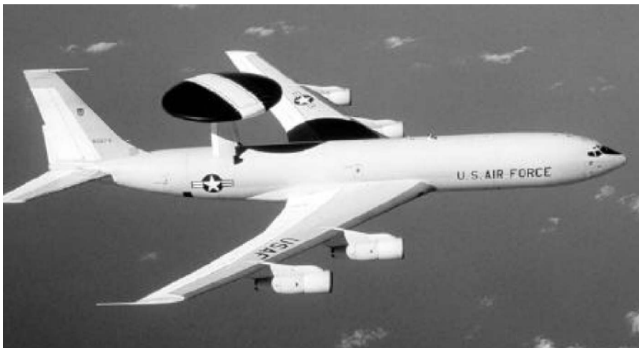
E-3 airborne warning and control system aircraft
