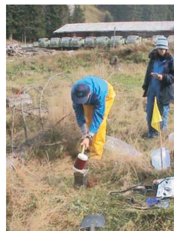
A large hammer is used to drive the soil profile plate into the ground
